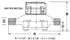
THE METER SHALL BE INSTALLED SO THAT IT IS EASILY ACCESSIBLE FOR FUTURE INSPECTIONS OR REPLACEMENT.
